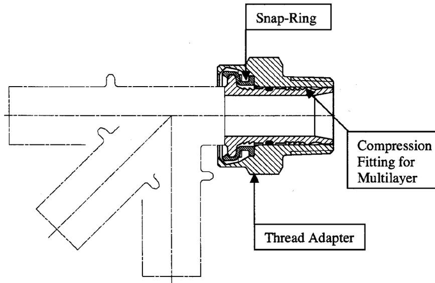
FIG. A1.1 Compression Fitting with Thread Adapter (and Snap-Ring) for Multilayer Pipe
